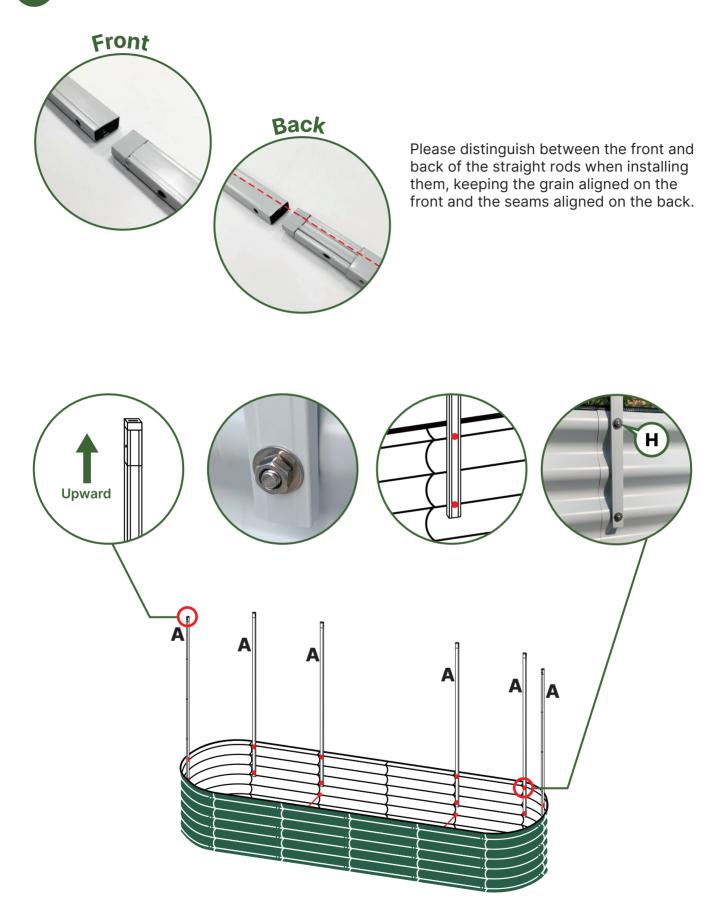
Fix the A-rods in the garden bed with an H-screws against the top two holes, with the narrower end of the A-rod toward the top.
