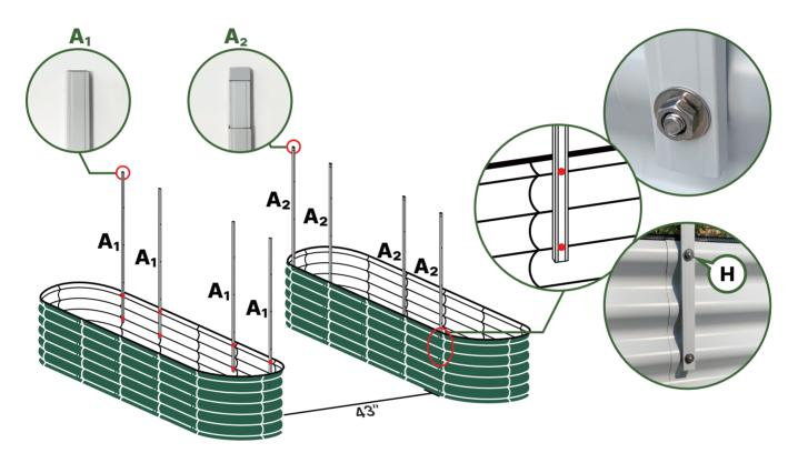
Fix four A1-rods to one of the garden beds with H-screws as marked in the diagram, with the narrower end of the rod facing upward. Fix four A2-rods to another garden bed with H-screws as marked in the diagram, with the narrower end of the rod upwards.
