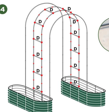
Installing the middle support rods, twelve D-rods, beginning with the hole closest to the garden bed and going to every other hole.
