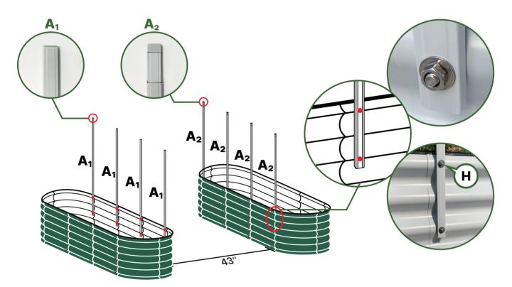
Fix four A1-rods to one of the garden beds with H-screws as marked in the diagram, with the narrower end of the rod facing upward. Fix four A2-rods to another garden bed with H-screws as marked in the diagram, with the narrower end of the rod upwards.
