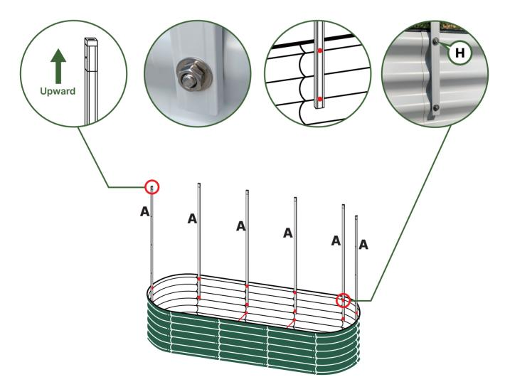
Fix the A-rods in the garden bed with an H-screws against the top two holes, with the narrower end of the A-rod toward the top.
