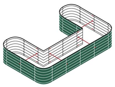
17 in.H  $\times$  8.5 ft.L  $\times$  5.5 ft.W Bracing Rod: 4  $\times$  2.5ft
