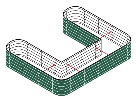
17 in.H  $\times$  8.5 ft.L  $\times$  7 ft.W Bracing Rod: 4  $\times$  2.5ft
