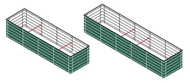
17 in.H  $\times$  6.5 ft.L  $\times$  2 ft.W Bracing Rod: 2  $\times$  2ft
