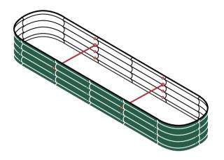
11 in.H  $\times$  8 ft.L  $\times$  2 ft.W Bracing Rod: 2  $\times$  2ft
