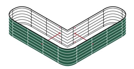
17 in.H  $\times$  7 ft.L  $\times$  7 ft.W Bracing Rod: 2  $\times$  2.5ft
