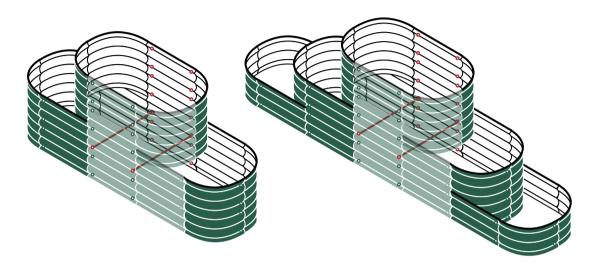
32 in.H  $\times$  6.5 ft.L  $\times$  2 ft.W Bracing Rod: 2  $\times$  2ft
