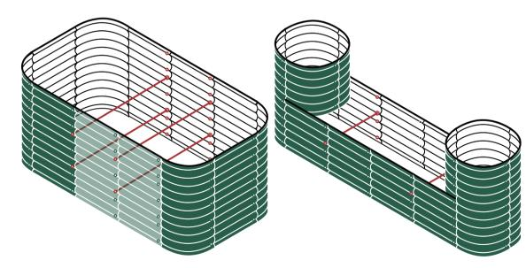
32 in.H  $\times$  6.5 ft.L  $\times$  3.5 ft.W Bracing Rod: 4  $\times$  (2+1.5)ft
