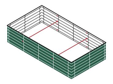
17 in.H  $\times$  6.5 ft.L  $\times$  3.5 ft.W Bracing Rod: 2  $\times$  (2+1.5)ft
