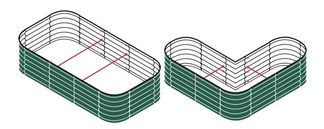
17 in.H  $\times$  6.5 ft.L  $\times$  3.5 ft.W Bracing Rod: 2  $\times$  (2+1.5)ft
