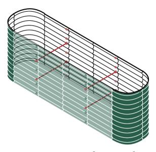
32 in.H  $\times$  8 ft.L  $\times$  2 ft.W Bracing Rod: 4  $\times$  2ft
