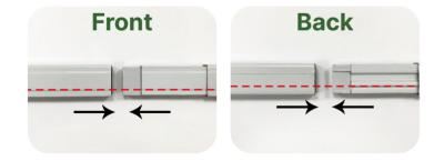
Connect eight B-rods and four C-rods as illustrated to form a oval, taking care to distinguish the front and back of each joint.
