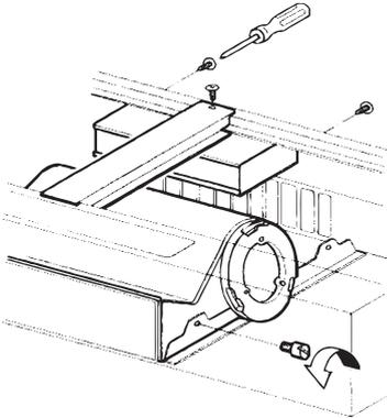
Remove the central support and control box by removing the screws indicated in figure. It is not necessary to remove the blower to perform this operation.
