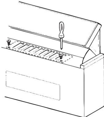
Attach the cover behind the exhaust grate with two silver screws 12e supplied with the rangehood.
