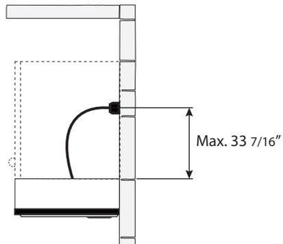
Do not use an extension cord. If the power supply cord is too short, have a qualified electrician install an outlet near the appliance.
