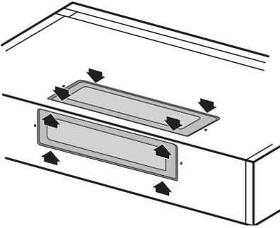
For Horizontal or Vertical ducting, the respective exhaust knockout must be removed. Each knockout is attached to the rangehood by four points. Using a flat blade screwdriver or utility knife, remove the exhaust knockout. Save this plate as it must be used to block the ductless exhaust grill. Figure shows the location of the knockouts for both horizontal and vertical. ONLY ONE must be removed.
