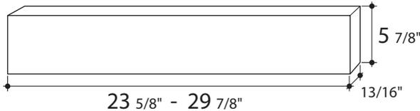
The front strip dimensions are shown above. If you wish to keep the frame of the front panel and only replace the glass panel, the dimensions follow:
