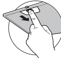
Replace the grease filters removed previously.
