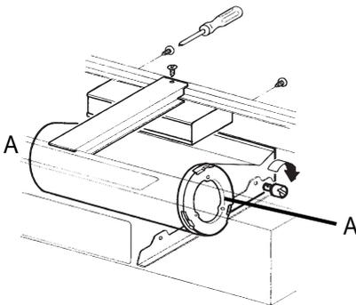
Remove the two black filter holders (**A**) in figure on each end of the blower by removing the 3 screws. Then Rotate the blower 180° so that the exhaust points out the front of the rangehood. Replace the black filter holders and the two thumb screws and tighten so that the blower is securely fastened inside the rangehood as indicated in figure. Reattach the control box and central support. Make sure that the wiring harness is concealed behind the central support.
