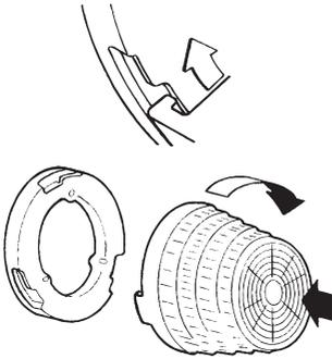
For ductless installations, Charcoal Filters are required and must be installed before the grease filters are replaced. The charcoal filters attach to both ends of the blower.
