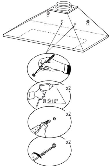
From inside the Hood body, mark the security hole, drill  $\varnothing 5/16"$  where marked, insert 2 wall plugs 11 in the holes and fix with 2 screws.
