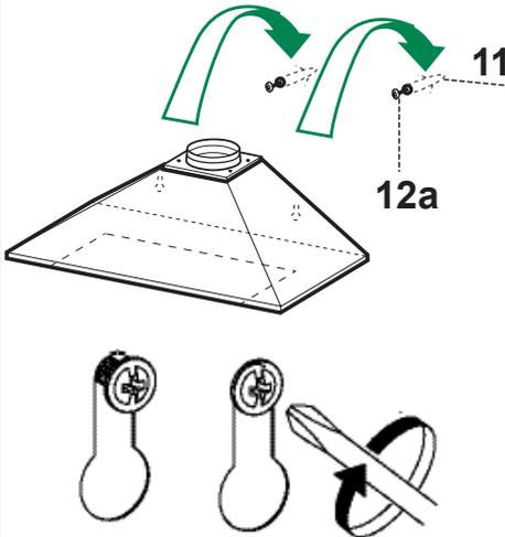
Hook the hood body onto the screws and screw completely.
