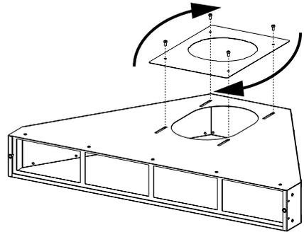
It is possible to slightly rotate or shift the final position of the flange. See figures on the right.
