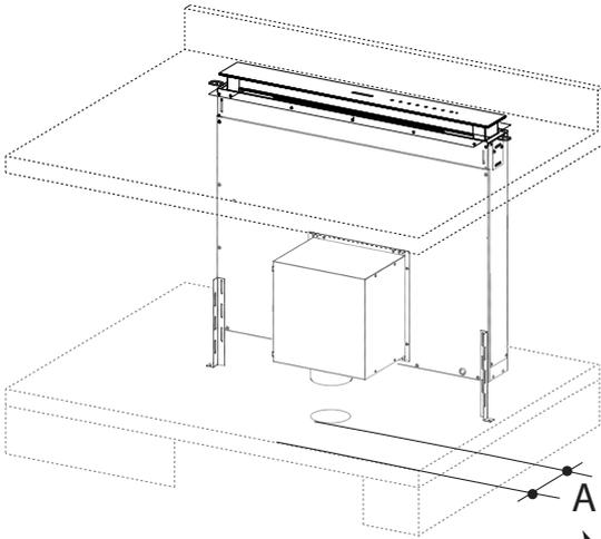
Measure the distance **A** from the hole to the cabinet external part, included the thickness of the cabinet.
