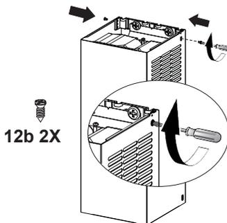
Secure the sides to the brackets by using the 2 screws 12b.
