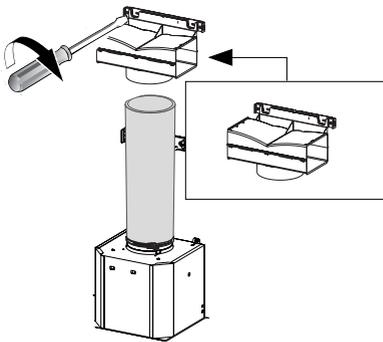
Fix the Ductless Diverter with two screws 12a supplied as shown.
