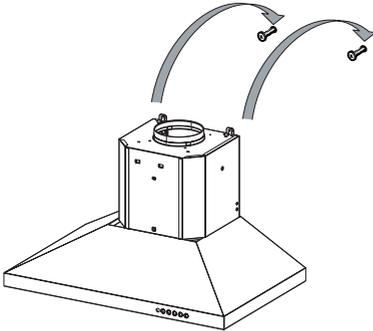
Hook the hood body onto the hood body fixing screws.
