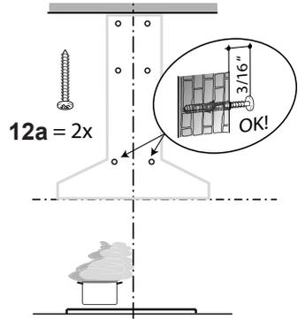
Insert not completely the two screws 12a supplied in the hood body fixing holes as shown.
