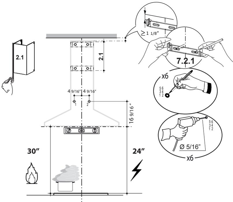
Draw a horizontal line where indicated at the bottom edge of the vent hood at the desired height above the cooking surface.
