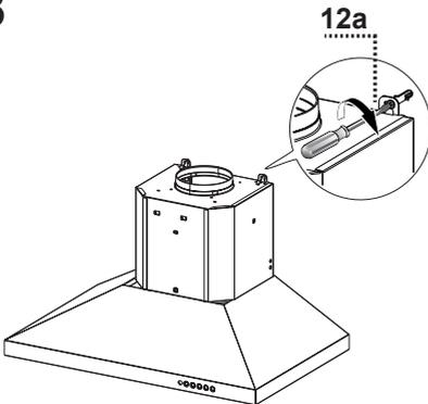
Tighten the 2 screws 12a as shown.
