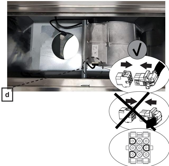
**3** Plug the power cable on the blower in the position E.
