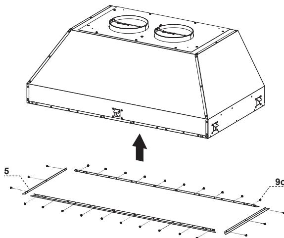
Follow step 1-2 to connect ducting, and test the electrical connection.
