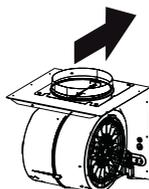
For a horizontal ducting installation the motor needs to be unsecured by first removing the 12 screws as shown.
