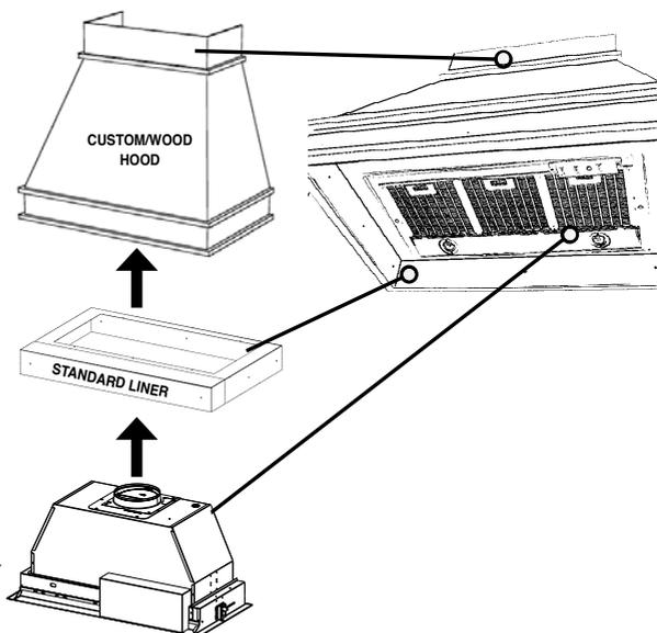
1. The custom/wood hood must have a sturdy base (3/4" plywood recommended) to accommodate the cut-out for the Inca HC SS. The base must be recessed to accommodate the height of the Liner (see **LINER DIMENSIONS** on Page 12). The Liner attaches to the bottom of the base using screws appropriate for the size and material of your custom/ wood hood. The Inca HC SS inserts into the cut-out in the Liner and base.
