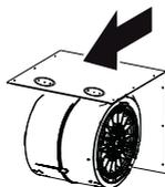
Once the blower is in place re-install the 12 screws to fasten the motor to the Insert Hood body.
