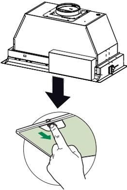
Remove the three filters from the Insert Hood before installing into cabinet.
