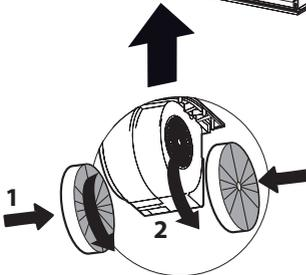
Attach each charcoal filter to the black grid on each side of the blower. Press the charcoal filter tightly to the black grid on the blower side and rotate the filter clockwise (towards the front of the insert hood) until it locks into place. Turn counterclockwise (towards the back of the insert hood) to remove.
