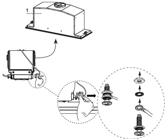
The Hood can be installed directly on the underside of the wall unit (Minimum 24" - 30" from the Cooking Surface).
