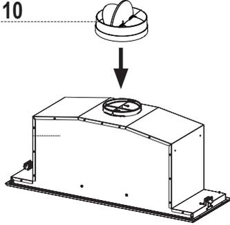
Install Damper that is included with the Hood before connecting to the ductwork.
