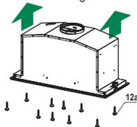
Insert the hood until the side supports snap into place.
