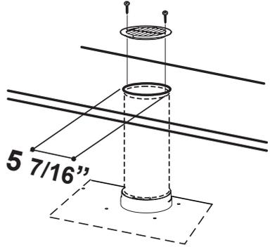
For Non-Ducted Recirculation venting route the ductwork to a location above the hood where the discharge is vented back into the room.
