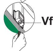
Open the filter cover panel by turning the specific knob.
