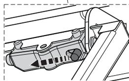
Screw the Frame into place using the 6 screws **12f**, reconnect the wires to the Connector and the Electrical ground cable (Yellow/Green) removed previously. Replace the metal grease filter and the Panel.
