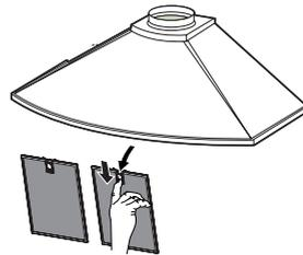
Replace the grease filters removed previously.
