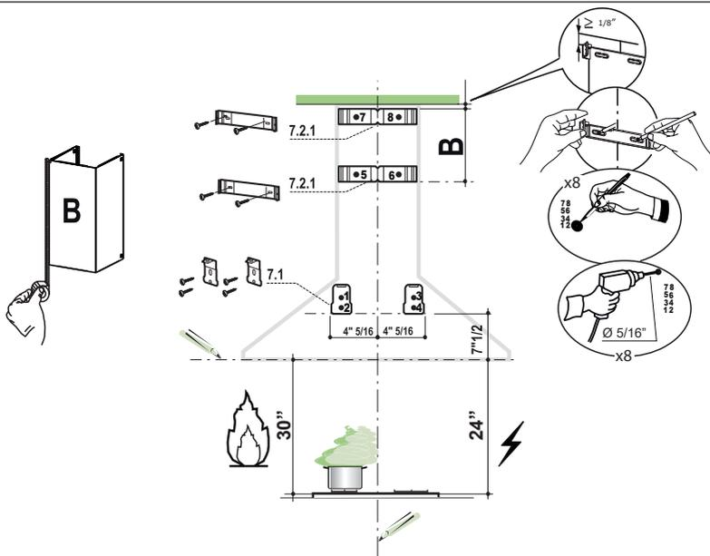
Place a Upper bracket 7.2.1 on the wall as shown about 1/8" from the ceiling or upper limit, aligning the centers(notch) with the vertical reference line and mark the wall at the centers of the holes in the bracket. Place the other bracket 7.2.1 on the wall as shown, below the first bracket, at the height of the upper chimney section supplied and aligning the centers (notch) with the vertical line.
