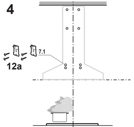
Fix the brackets 7.1 using the 12a screws supplied in the hood body fixing holes as shown.
