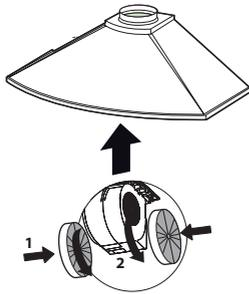
grid on the blower side and rotate the filter clockwise (towards the front of the hood) until it locks into place. Turn counterclockwise (towards the back of the hood) to remove.
