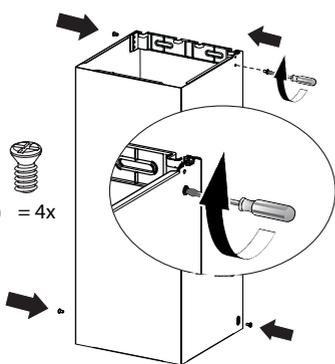
Secure the sides to the brackets by using the 4 screws 12b.
