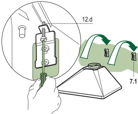
Screw the two screws 12d supplied onto the brackets 7.1.
