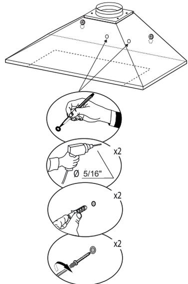
From inside the Hood body, mark the security hole, drill  $\varnothing 5/16''$  where marked, insert 2 wall plugs in the holes and fix with 2 screws 12a.
