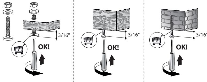
Use only screws and small parts in support of the hood.
