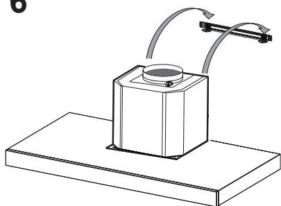
Hook the hood body onto the hood body fixing bracket 7.3.
