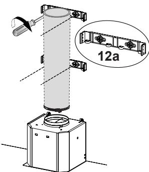
Install the 2 fixing brackets 7.2.1 to the middle and upper holes and secure with screws 12a as shown.
