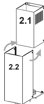
Slightly widen the two sides of the the lower chimney hood and hook them between the upper section and the wall, making sure that they are properly housed.
