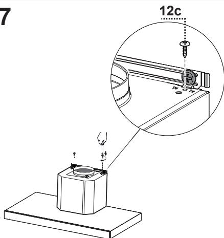
Tighten the 2 screws 12c as shown.
