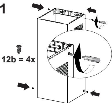
Secure the sides to the brackets by using the 4 screws 12b.
