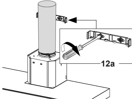
Fix the lower Bracket 7.2.1 with two screws 12a supplied as shown.
