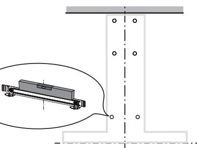
Use a level to insure that Fixing Bracket is level and then fully secure the two screws.
