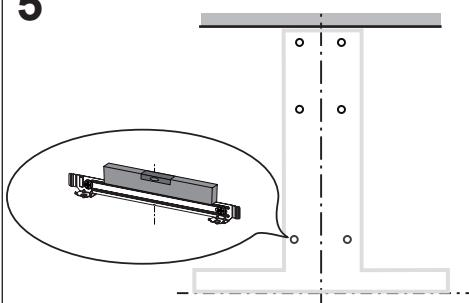
Use a level to insure that Fixing Bracket is level and then fully secure the two screws.
