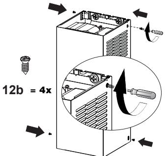
Secure the sides to the brackets by using the 4 screws 12b.
