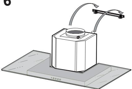
Hook the hood body onto the hood body fixing bracket 7.3.
