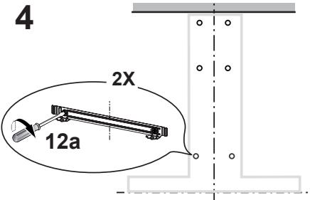
Insert the two screws 12a supplied with the hood into the Fixing Bracket as shown and do not tighten all the way to wall leaving  $3/16"$  of the screw heads exposed.
