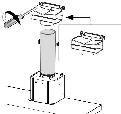
Fix the Ductless Diverter with two screws 12a supplied as shown.
