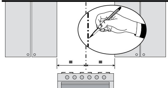
Draw a vertical line on the supporting wall as high as practical, at the center of the area in which the hood will be installed.
