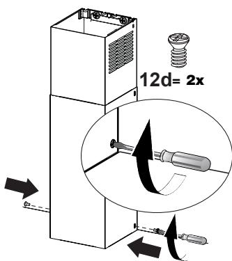
Fix the the lower chimney hood laterally to the hood body using the 2 screws 12d supplied.
