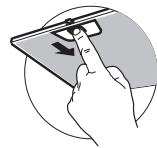
Remove the filters one at a time by pushing them towards the back of the board and pulling down at the same time.
