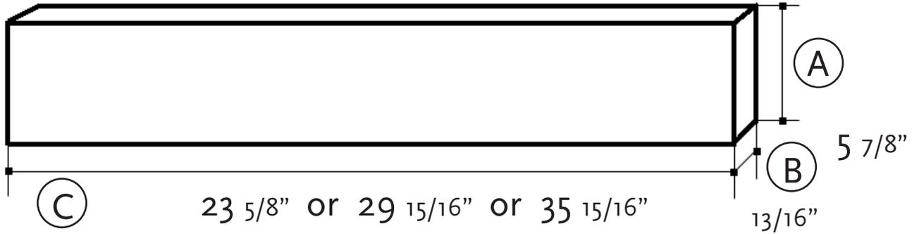
\* If you wish to keep the frame of the front panel and only replace the glass panel, the dimensions are as follows:
