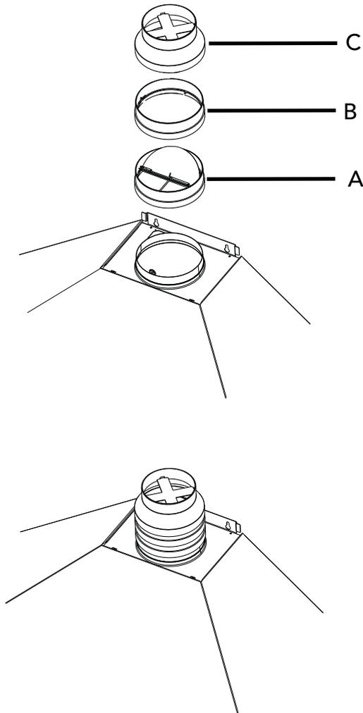
**NOTE: CFM REDUCER KIT CONVERTS THE CFM TO UNDER 300 CFM FOR USE IN MAKE UP AIR ENVIRONMENTS**
