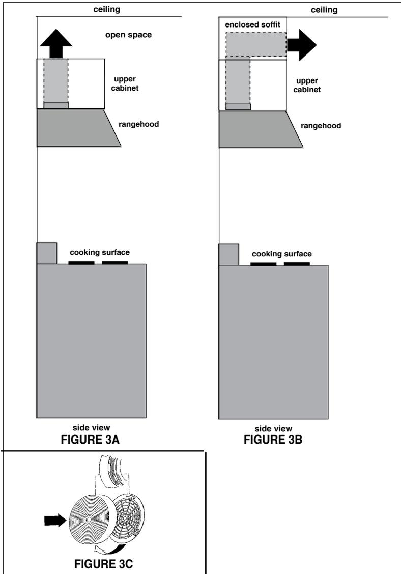
**NOTE:** it is recommended that professional style cooking always be vented to the outside; for recirculating installations, some duct work is required to exhaust the unit out of the cabinet. For 48" model, order 2 kits, one for each motor.
