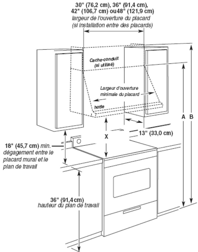
A. 84" ; MINIMUM POUR DES INSTALLATIONS AVEC LA VERRIÈRE SEULEMENT B. 96" ; MINIMUM POUR LES COUVERTURES FACULTATIVES DE CONDUIT D'INSTALLATIONS
