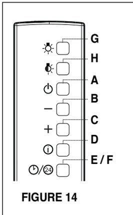
The hood can be operated from the control panel located on the right hand side of the hood or from the remote control. **FIGURE 13** is an illustration of the control panel and **FIGURE 14** is the remote control illustration. On the remote control key E and F are controlled with one button. Press the button once for function key "F" - 30 minute shut down". Hold for 2 seconds for function key "E" - 24 hr function.
