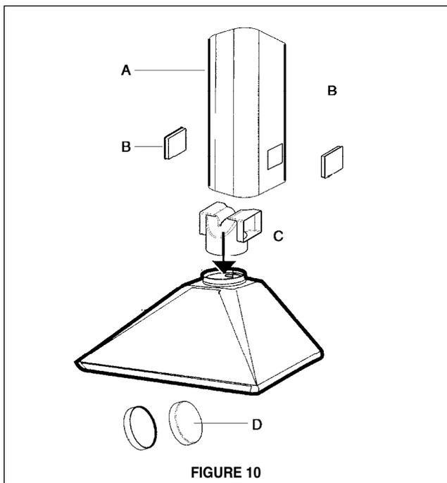
Once the LOWER CHIMNEY DUCTLESS with holes is installed, the VENT GRIDS (B) are inserted into the holes (FIGURE 11).
