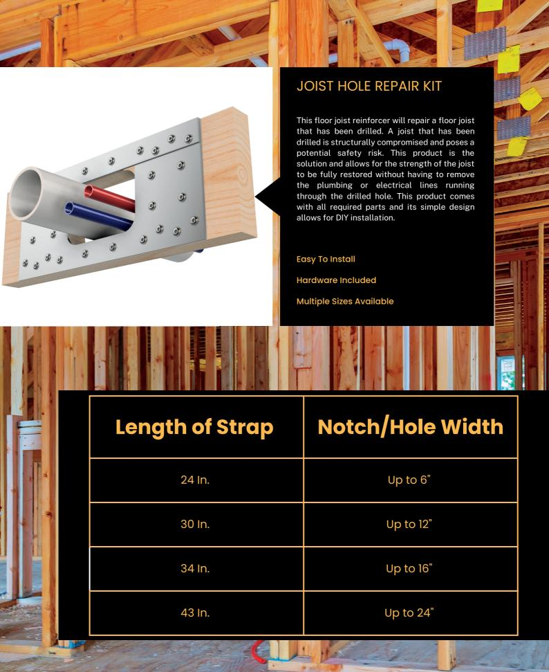
\*Minimum of 9 inches is required on each side of the notch for the screwed area of the strap to fit.
